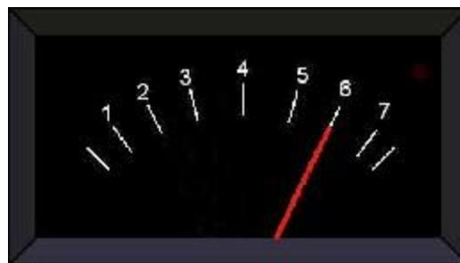
Slika 1.14 PPM (Peak Program Meter) metar.
